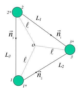
It is best to think of LISA as a closed array of six one-way delay lines between the test masses. This approach allows one to construct several interferometric data combinations. It offers advantages in hardware design, in robustness to failures of single links, and in redundancy of data [3-5].
